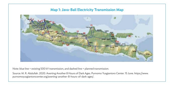
JABODETABEK and Bali are connected to the transmission network of the Java/Bali power system. This transmission network consists of overhead lines measuring hundreds of kilometers. JABODETABEK is connected with both 500-kilovolt and 150-kilovolt lines. In the central Jakarta area, underground 150-kilovolt cables transport the electricity in bulk to the dense load centers. Bali is only connected with 150-kilovolt lines, although a 500-kilovolt connection is penciled in PLN's plans.
